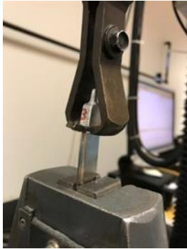
Pull testing of Al-Cu rotor bar
